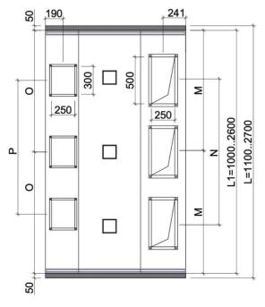
Note: The following data refers to the dimensions of the basic module hood. The actual hood can be assembled from the basic module hoods, which facilitates later transportation and on - site operation.
